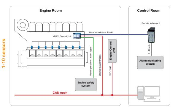
sensors ensure that the crankcase is monitored.
